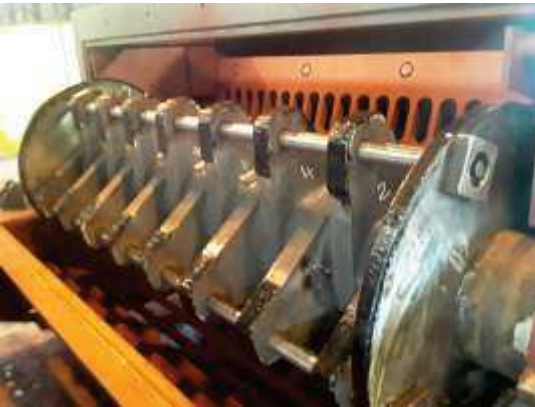
Hard face welding used on the rings
