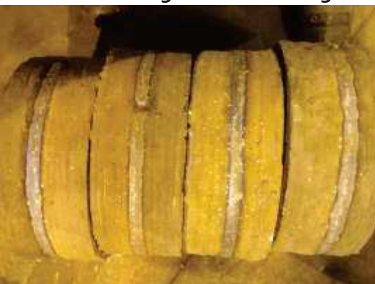
Hard face welding used on the rings
