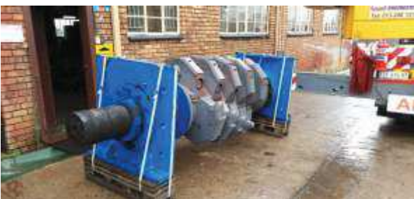
Pick shaft refurbished at the workshop And ready to go
